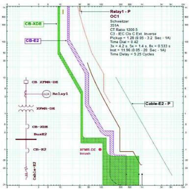
If the devices are not co-ordinated and properly set, the circuit breakers might demonstrate nuisance tripping or may not trip at all in the event of a disturbance/ fault. Also some healthy feeders might face power outage in the event of nuisance tripping. This might hamper critical loads from proper functioning
